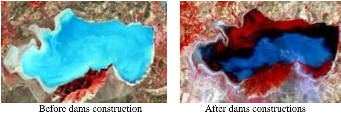
Figure 10: Lake Ichkeul, Tunisia. The lake badly deteriorated as the result of the construction of three dams on rivers supplying it and its marshes. The dams cut off almost all inflow of fresh water, causing a destructive increase in the salinity of the lake and marshes. (Source U.S./Japan ASTER Science Team and NASA/GSFC/METI/ERSDAC/JAROS)
